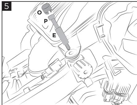
**Replace the original filter cover screws with the screws (P), the bushings (E) and the caps (O), as shown in figure. Repeat the process on the other side.**
