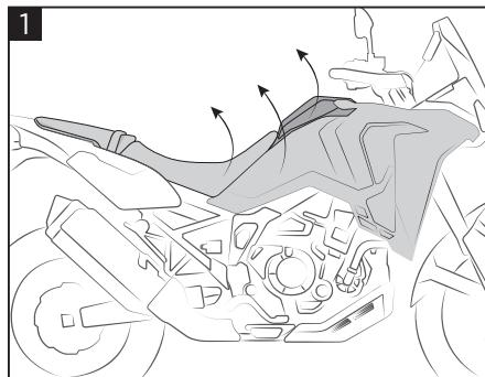
**Remove the original radiator shrouds, seat and tank.**
