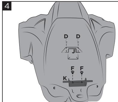
**Apply the brackets (J) and (K) using the screws (D) and (F).**
