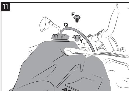
**Replace the original screw with the provided bushing (Y) and screw (F). Insert the gas' hose in the cap.**
