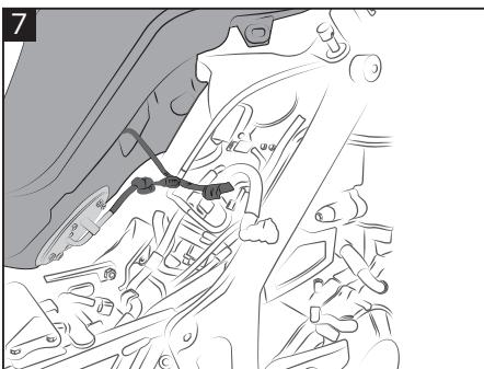
**Connect the outlets and place the fuel tank on the bike.**
