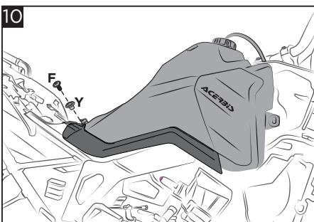
**Place the plastic and secure it using the provided bushing (Y) and screw (F). Repeat the operation on the other side. Then remount radiator shrouds and seat.**
