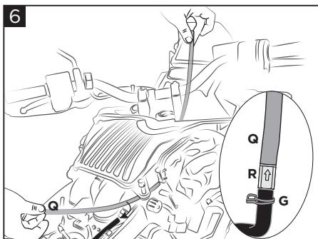
**Pull the hose (Q) through as shown in figure and connect it to the carbon canister gas' original hose using the valve (R) and the clips (G).**
