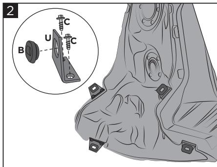
**Apply the four angled hose connectors (U) using the screws (C), then insert the rubber pads (B) as shown in figure.**
