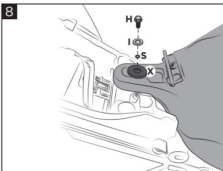
**Place the provided bushing (S) and the original washer (I) and the screw (H) inside the rubber pad (X).**
