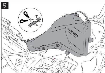
**Cut the biadhesive velcro (T) and paste it on the points shown in figure, on both sides.**
