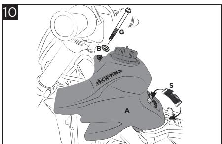
**Tighten the Acerbis fuel tank (A) using washer (B) and screw (G) and hook with the rubber band (S), paying attention to hook it first on the tank's bracket and then on the bike's frame.**
