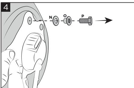
**Remove washers (N), bushings (O) and screws (P).**
