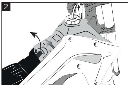
**Unhook the rubber band (S), untighten the original screw and remove the original fuel tank.**
