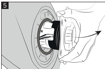
**Remove the original pump (L) and O-ring (R).**
