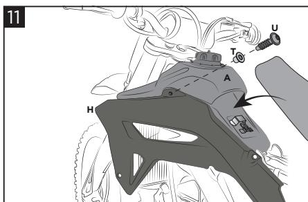
**Assemble the radiator shrouds (H) using washer (T) and screw (U). Then remount the saddle.**
