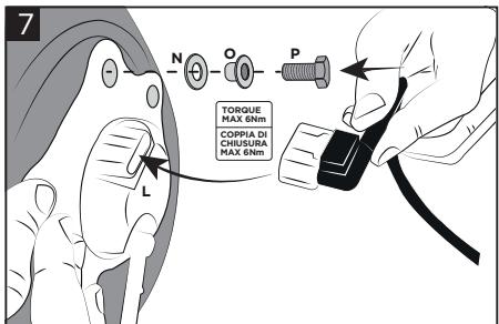
**Screw the pump trough washers (N), bushings (O) and screws (P) and connect the systems. ATTENTION: when tightening maximum torque spec 6Nm.**
