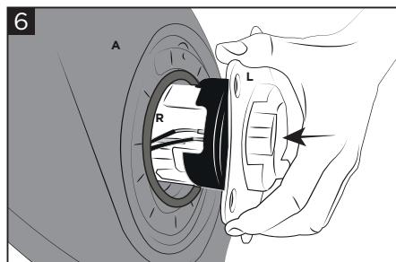
**Insert the O-ring (N) in its seat on the Acerbis fuel tank (A). Insert the original pump (L) on the Acerbis fuel tank (A).**
