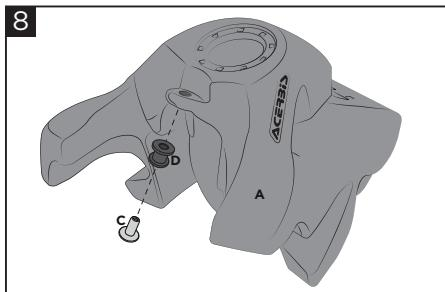
**Insert grommet (D) ad bushing (C) in the hole.**
