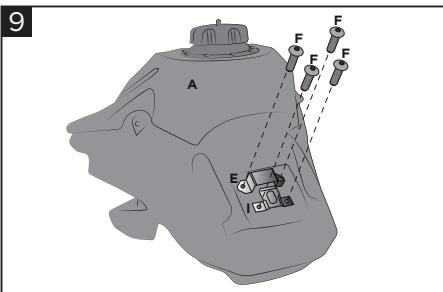
**Mount the brackets (E) and (I) through screws (F).**
