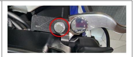
**Step 3:** Pull the lever outwards to remove it from the motorcycle.
