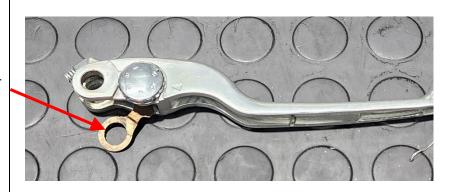
**Step 7:** Pull the adjuster knob out upwards.
