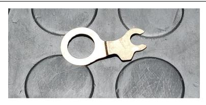
**Step 10:** Ensure that the copper plate hole aligns with the rest of the lever's inner components, before you push/tap the copper bush back into position. Check that the handguard holes align perfectly with the lever when installing the Wild@Heart lever, otherwise the bolt will not turn in completely.
