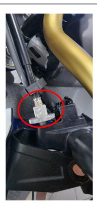
Step 2: Undo the clutch lever by loosening the indicated bolt using 2 x 10mm spanners. One spanner at the top of the bolt and the other at the associated bottom nut.
