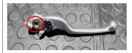
**Step 5:** Remove the inner component as per the photo. Make sure not to lose the spring.
