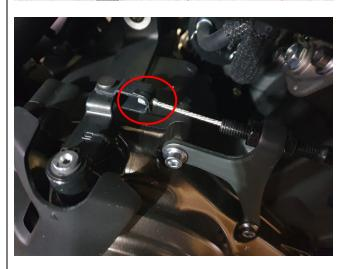
**Step 2:** Unscrew the bottom nut holding the clutch lever in place using a 10mm spanner.
