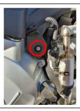
**Step 5:** Unhook the clutch cable by grabbing the cable with a longnose pliers.
