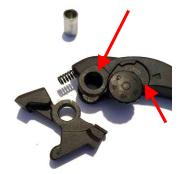
**Step 4:** Slide the adjuster knob out of the lever but pay attention as it is spring loaded at the bottom. If spring is stuck pull it out with the longnose pliers. Rebuild the components onto the Wild@Heart lever and install on the bike. Make sure the adjuster knob is set to no.1 and the spring is located positively into the dedicated areas. If the bush struggles to push through clean the bush and inside of the holes with a bit of sanding paper if necessary.
