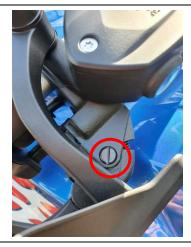
**Step 3**: First set the adjuster knob to setting no.1 then use a 10mm drill bit and a mallet to tap out the indicated bush – pay attention not to lose the inside spring.
