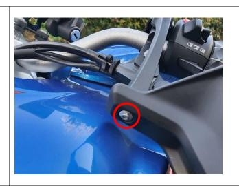
**Step 2:** Pull the handguards support bracket outwards to gain access to the lever bolt.
