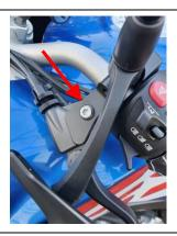
**Step 3:** Turn adjuster knob lock nut out completely clockwise and the adjuster knob all the way anti-clockwise.
