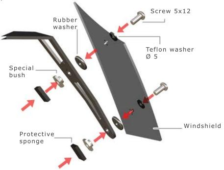
STEP 2: COMPLETE THE MOUNTING PROCESSING FIXING THE WINDSHIELD/SCREEEN BRACKET ON THE STEERING PLATE USING THE SCREWS
