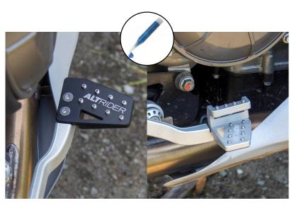
(3) Remove Factory brake pedal. If you have only the enlarger use included M5 fasteners to attach the enlarger. Use thread locker, tighten to 4.4Nm.
