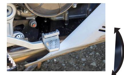
(4) Check brake pedal movement to be sure there is no interference with other parts of your bike.
