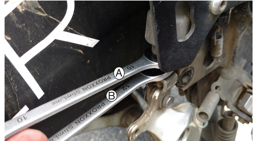
⑥ Use 10mm spanner to hold the master cylinder shaft still. (A) Use 12mm spanner to loosen the jam nut that is against the yoke. (B)
