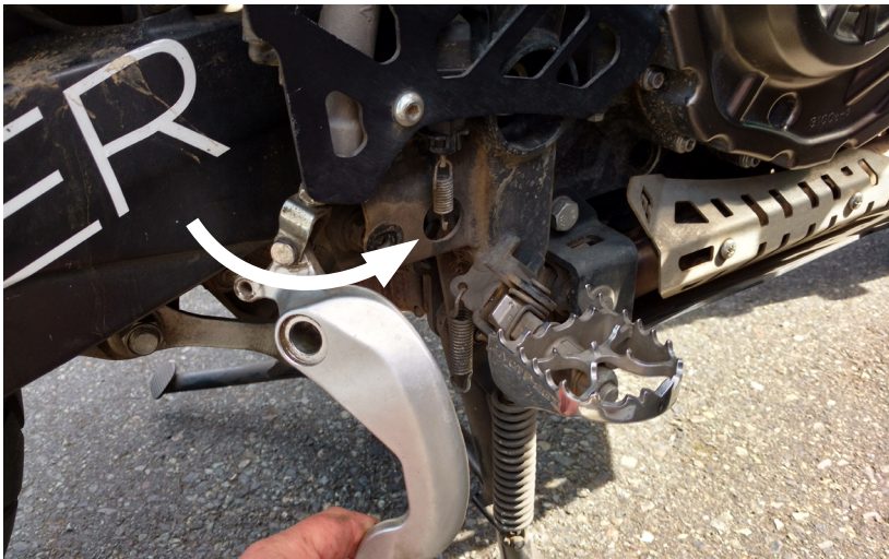
⑦ Hold plunger still (do not rotate). Turn entire brake lever to move the yoke up or down on the shaft. This will set your new lever height. Spinning the yoke up the shaft will move your brake lever tip downwards.
