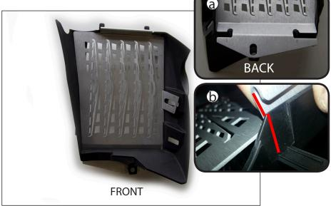
Fit each radiator guard into its respective shroud like pictured about. Make note of how they fit together be examining the shot of the assembly from behind (a) and where the radiator guard clips on to the top. If unsure how to line guard up to shroud, use diagram (b) and line up the two red lines.
