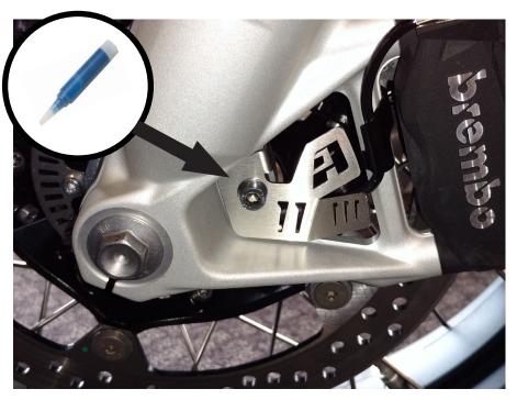
Apply one drops of thread-locker to the ends of the M6 x 20mm long screw provided. Use the 5mm hex Allen tool to install the new guard with the screw and two M6 stainless steel washers. One washer on the backside of the guard, one washer under the screw head. Tighten to 6Nm.
