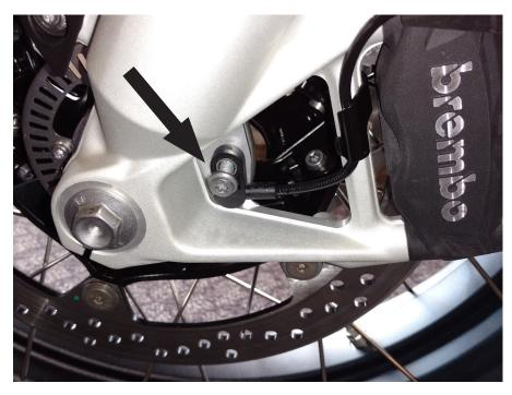
Remove the T30 torx fasteners from the ABS Sensor. **!CAUTION!** If your ABS sensor wire is routed differently than shown, do not install this guard.
