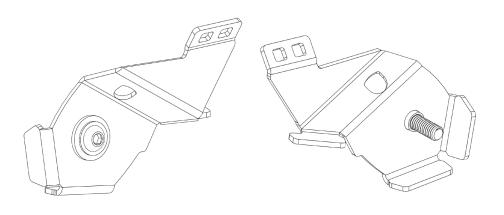
Place plastic washer, spacer, and switch guard on supplied M6 x 20 button head screw as shown. Then add loctite to the last few threads of the screw. Avoid getting loctite on the spacer and plastic washer.
