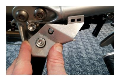
3 Screw side stand switch in place. Attach zip ties around frame.
