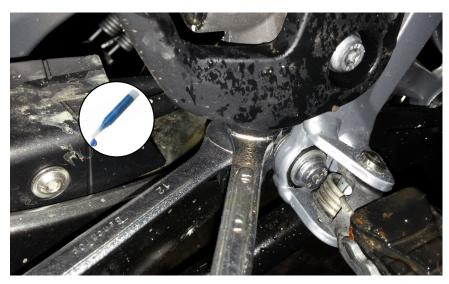
Hold plunger still with 10mm wrench. Apply a drop of loctite to the threads below the jam nut. Spin jam nut down until it contacts the yoke. Tighten against yoke.
