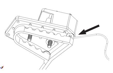
Place DualControl onto your bike's brake lever. Be sure the lever is seated in the groove on the underside of the Enlarger. Be sure the Brake Snake is on top of the lever in the position shown (arrow).
