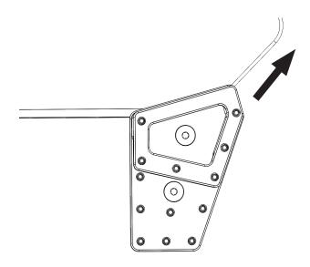
6 Correct Brake Snake cable location. Should be on top of lever, under enlarger.
