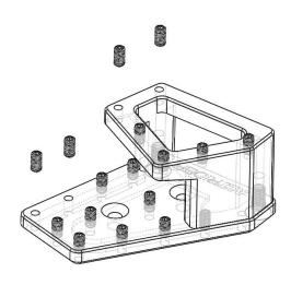
(2) Install M4 x 8mm Grip pins, using 2mm Allen driver. Usea a small dot of thread locker on each pin. Total number and placement is up to you. Tighten snug, but be careful not to strip the tool.
