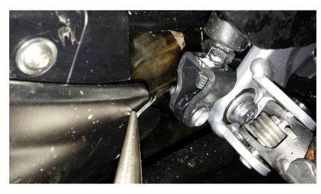
6 Reinsert the pin and check brake lever is at desired height. Reinstall washer and cotter pin.
