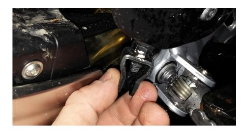
(5) Holding the plunger still, spin the yoke so it moves higher up the plunger, toward the master cylinder.
