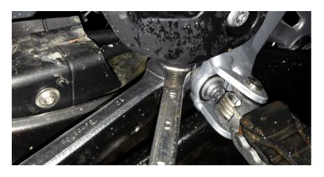
② Use a 10mm and 12mm open end wrench. With the 10mm wrench on top, hold the plunger still. There are wrench flats on the plunger right near the rubber boot where it enters the master cylinder. The plunger must not spin, this preserves the correct internal adjustment. While holding the plunger, use the 12mm wrench to loosen the jam nut.
