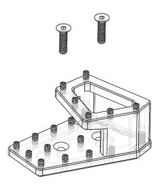
(3) Place two (2) M5 x 20mm flat head screws through enlarger plate.
