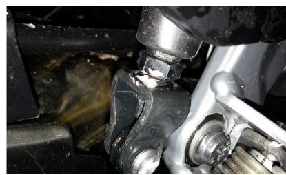
Spin the jam nut higher up the plunger rod, toward the master cylinder. Do not spin the plunger rod itself.
