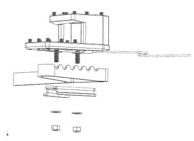
Attach DualControl to brake pedal with metal plate, washers, and lock nuts. Use M3 allen on screws and 8mm socket on locknuts and tighten snug.
