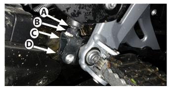
Locate the master cylinder and plunger connected to the brake pedal, direcly behind the right side foot peg. Note parts: (A) plunger shaft wrench flats.
