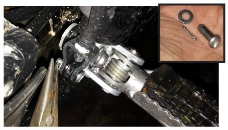
Pull the small cotter pin. Pull the washer and the pivot pin that connects the yoke to the plunger.
