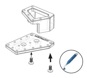
If your kit is equipped with the full DualControl Enlarger + Riser, install the riser now. Place a drop of thread locker on each of the two (2) M5 x 12 flat head screws and use an M3 Allen to tighten the parts together.
