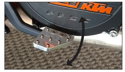
(2) Check brake pedal movement to be sure there is no interference with other parts of your bike. For optimal performance adjust your brake lever height to your preference. Refer to manufacturer's instructions for your specific bike to complete that adjustment.
