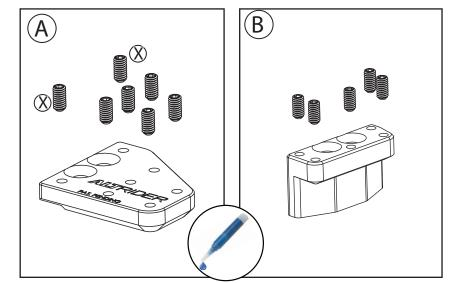
$(\mathcal{I})$  (A) Install M4 x 8mm Grip pins, using 2mm Allen driver. Use a small dot of thread locker on each pin. Tighten snug, but be careful not to strip the tool. If using optional riser, do not install the two pins marked X. (B) Install the grip pins in the riser part.
