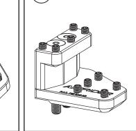
Attach AltRider DualControl to brake lever arm using M5 flat head screws. (3) Use a drop of threadlocker on each screw. Tighten to 4Nm.
