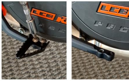
Remove the OEM brake pedal tip. Use a T30 or T25 torx, depending on (1)which model motorcycle you are working on.
