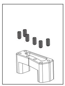
(A) If your kit is equipped with the optional Riser, install the grip pins in the riser now. Then apply drop of thread locker to the two M5 x 12mm flat head screws, and attach to the enlarger base.
