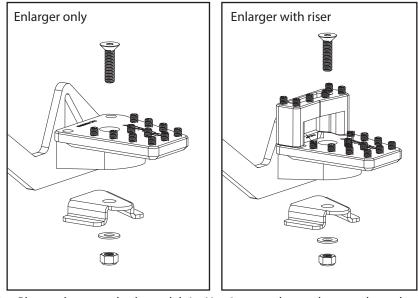
Place enlarger on brake pedal tip. Use 8mm socket tool to attach steel lower plate with M5 washer and M5 locknut. Tighten to 4.4Nm.
