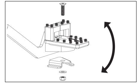
(4) Check brake pedal movement to be sure there is no interference with other parts of your bike. If the riser is installed, adjust your brake pedal height so that in the seated position you are using the enlarger, while in the standing position you will use the riser. Adjust your pedal height using the manufacturer's instructions to ensure correct procedure. It is important to set the correct free play to avoid caliper drag and potential brake failure.
