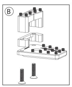
(A) If your kit is equipped with the optional Riser, install the grip pins in the riser now. (B) If your kit also has the spacer block, place it between the enlarger and riser. (All) Then apply drop of thread locker to the two M5 x 12mm (or 22mm if using the spacer) flat head screws, and attach to the enlarger base.
