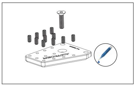
Install M4 x 8mm Grip pins, using 2mm Allen driver. Use a small dot of thread locker on each pin. Total number and placement is up to you. Tighten snug, but be careful not to strip the tool. Insert the M5 x 20mm flathead screw through the enlarger.
