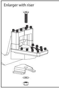
Place enlarger on brake pedal tip. Use 8mm socket tool to attach steel lower plate with M5 washer and M5 locknut. Tighten to 4.4Nm.
