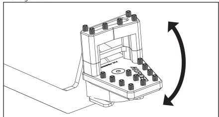
Check brake pedal movement to be sure there is no interference with other parts of your bike. If the riser is installed, adjust your brake pedal height so that in the seated position you are using the enlarger, while in the standing position you will use the riser. Adjust your pedal height using the manufacturer's instructions to ensure correct procedure. It is important to set the correct free play to avoid caliper drag and potential brake failure.
